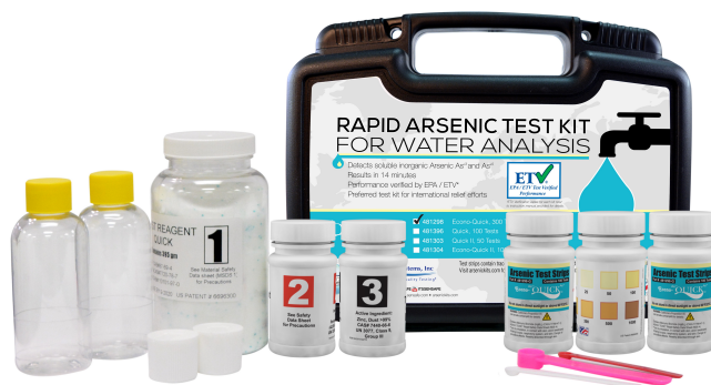
Figure 1: Example of a rapid arsenic test kit for drinking water analysis [2].
