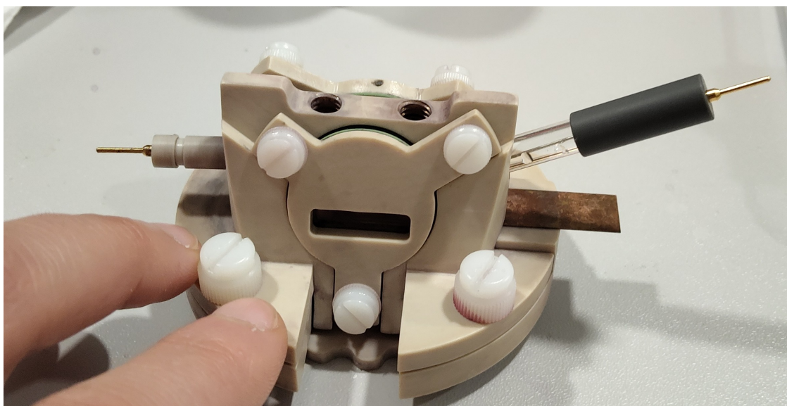
Figure 5: Ellipsometry EC angle-of-incidence 70° measurement cell used in this work.
